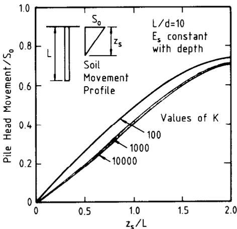
Fig. 19. Elastic solutions for pile movement in expansive soil—uniform pile diameter
