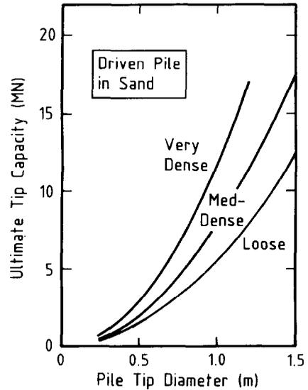
Fig. 39. Design chart for ultimate tip capacity of driven piles in sand
