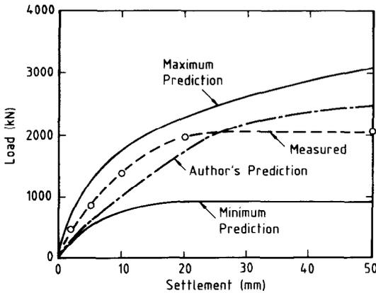
Fig. 53. Predicted and measured load-settlement behaviour pile 1
