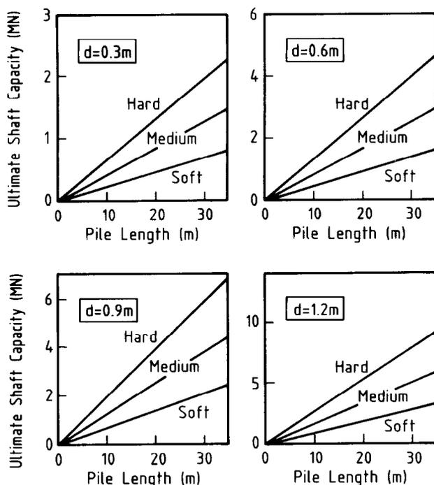
Fig. 37. Design charts for ultimate shaft capacity of driven piles in clay: (a)  $d = 0.3\text{ m}$ ; (b)  $d = 0.6\text{ m}$ ; (c)  $d = 0.9\text{ m}$ ; (d)  $d = 1.2\text{ m}$
