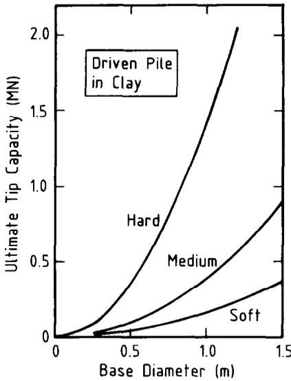
Fig. 38. Design chart for ultimate tip capacity of driven piles in clay
