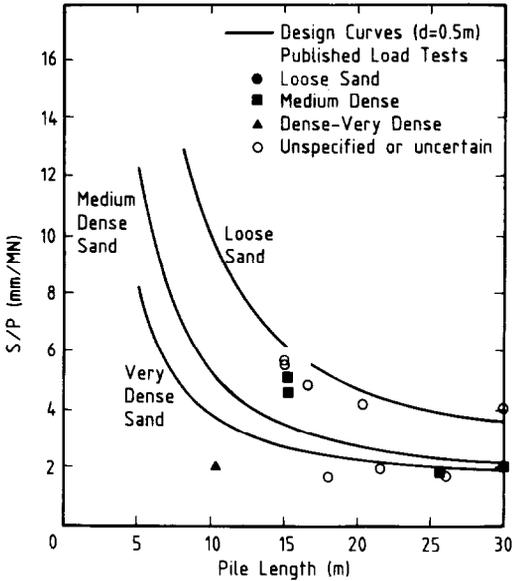
Fig. 32. Design chart for settlement of driven piles in sand (diameter =  $0.5 \pm 0.1$  m)
