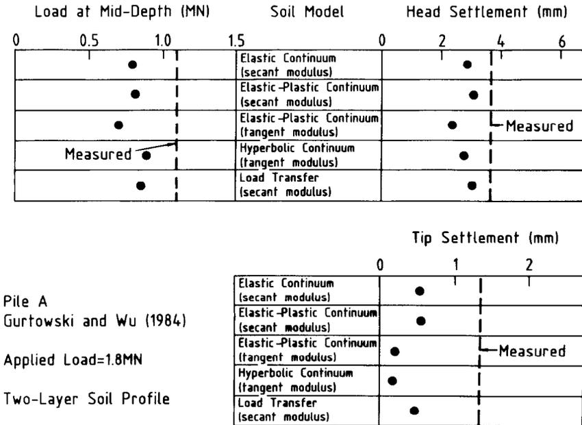
Fig. 42. Influence of soil model on predicted behaviour of single pile
