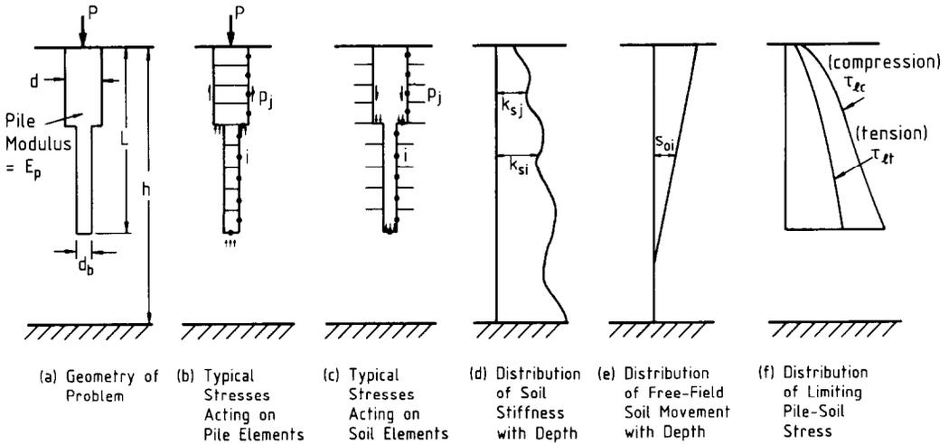
**Fig. 1. Basic problem of single axially loaded pile: (a) geometry; (b) stresses acting on pile elements; (c) stresses acting on soil elements; (d) distribution of soil stiffness with depth; (e) distribution of free-field soil movement with depth; (f) distribution of limiting pile-soil stress**
