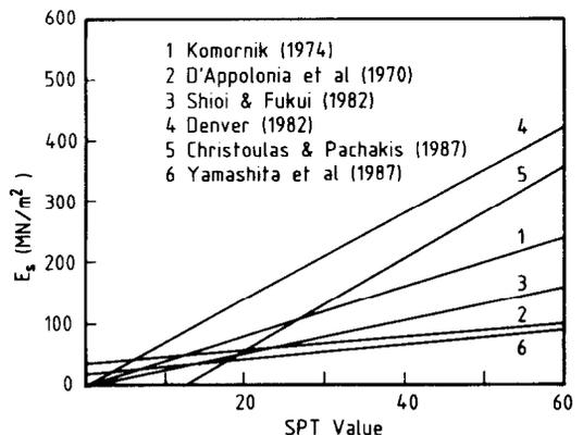
Fig. 29. Comparison between correlations for soil modulus driven piles in sand
