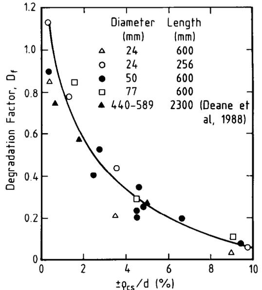
Fig. 21. Effect of normalized cyclic slip displacement on  $D_r$  with different pile diameters (after Lee, 1988)
