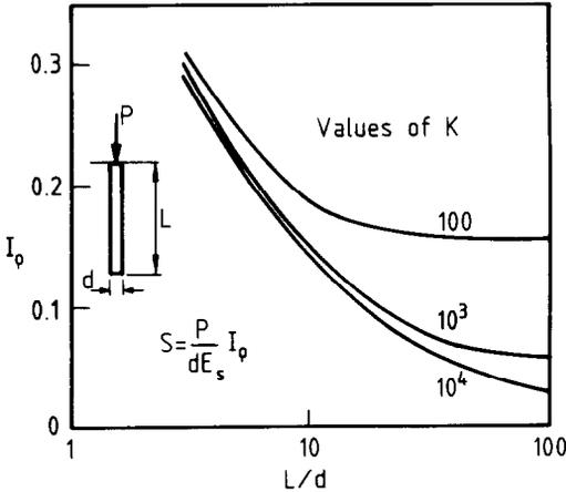
Fig. 8. Influence of dimensionless parameters  $L/d$  and  $K$  on settlement. Single friction pile in homogeneous soil
