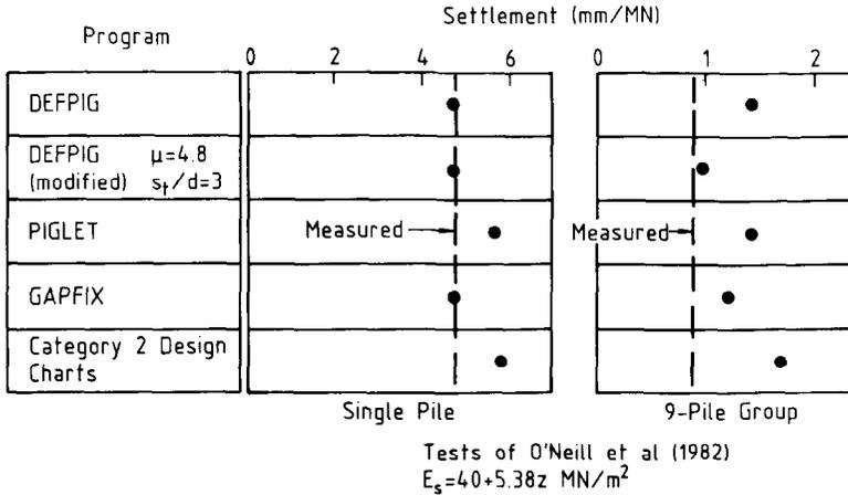
Fig. 47. Effect of analysis method on single pile and group settlements
