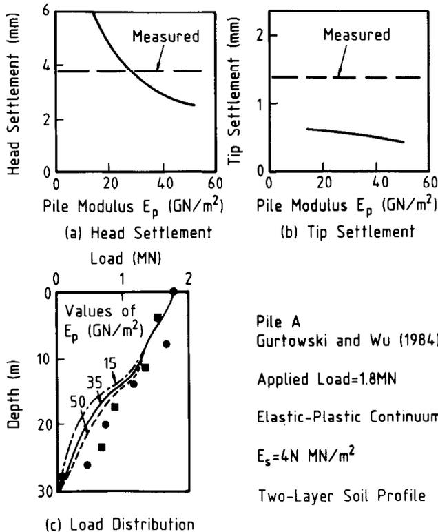
**Fig. 45. Influence of pile modulus on behaviour of single pile: (a) head settlement; (b) tip settlement; (c) load distribution**
