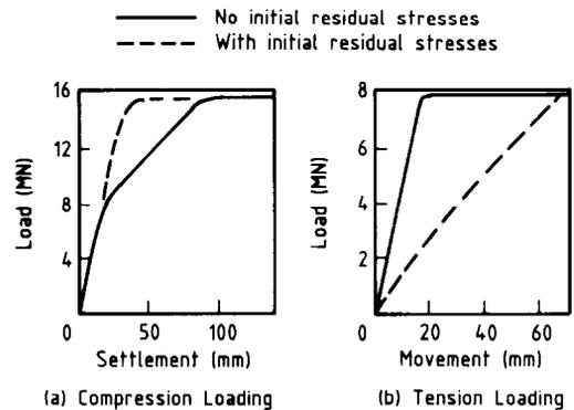
**Fig. 12. Effect of residual stresses on load-deflection behaviour pile in sand (Poulos, 1987): (a) compression; (b) tension**
