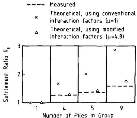
Fig. 48. Theoretical and measured group settlement behaviour (Tests of O'Neill *et al.*, 1982)
