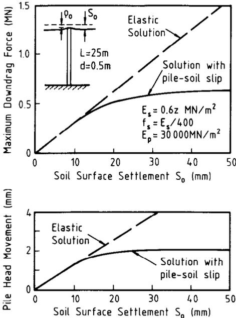
**Fig. 17. Influence of pile-soil slip on dowdrag force and pile movement**
