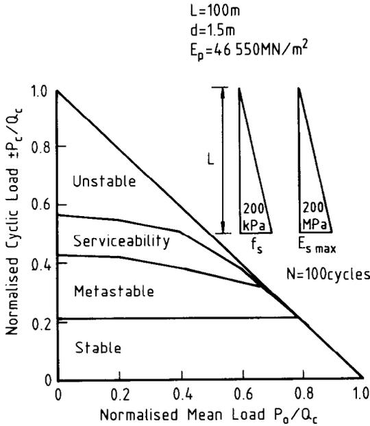
Fig. 22. Typical cyclic stability diagram for offshore pile;  $N = 100$  cycles (Lee, 1988)
