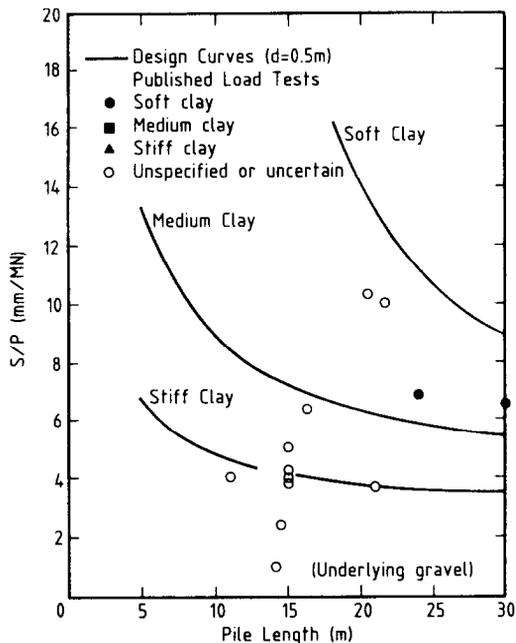
Fig. 31. Design chart for settlement of driven piles in clay (diameter = 0.5 ± 0.1 m)
