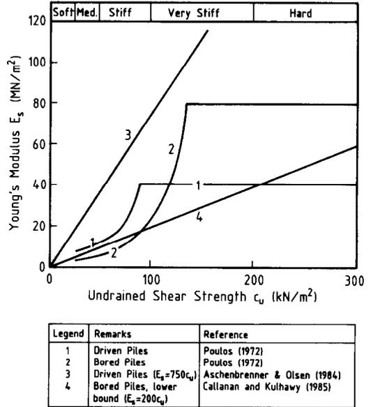
Fig. 28. Correlations for soil modulus for piles in clay (after Callanan & Kulhawy, 1985)
