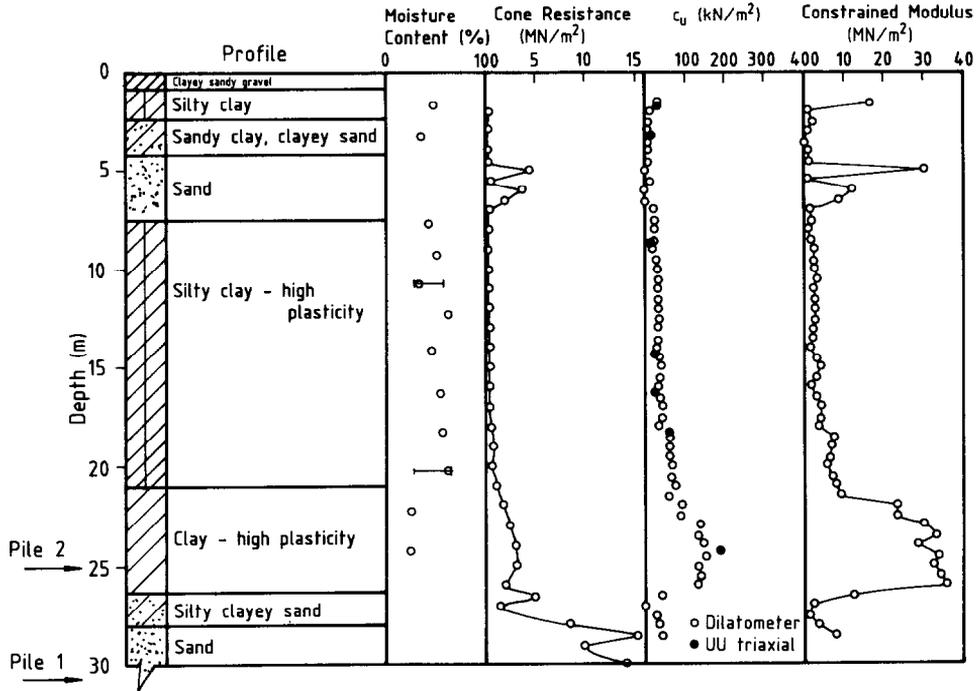
Fig. 52. Geotechnical data at Hemmant test pile site
