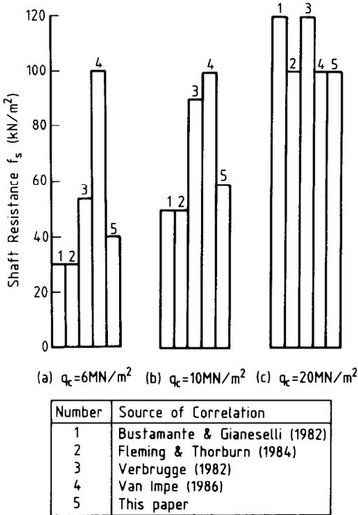
Fig. 27. Example of variations between correlations for shaft resistance against CPT-driven piles in sand: (a)  $q_c = 6 \text{ MN/m}^2$ ; (b)  $q_c = 10 \text{ MN/m}^2$ ; (c)  $q_c = 20 \text{ MN/m}^2$
