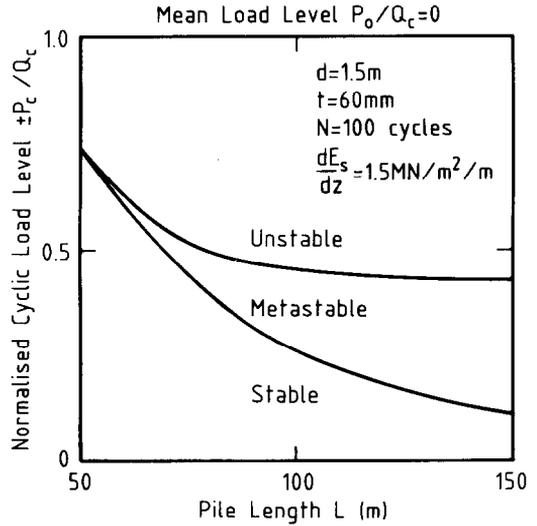
Fig. 23. Effect of pile length on stability diagram zone boundaries. Driven pile in clay (Poulos, 1988b)
