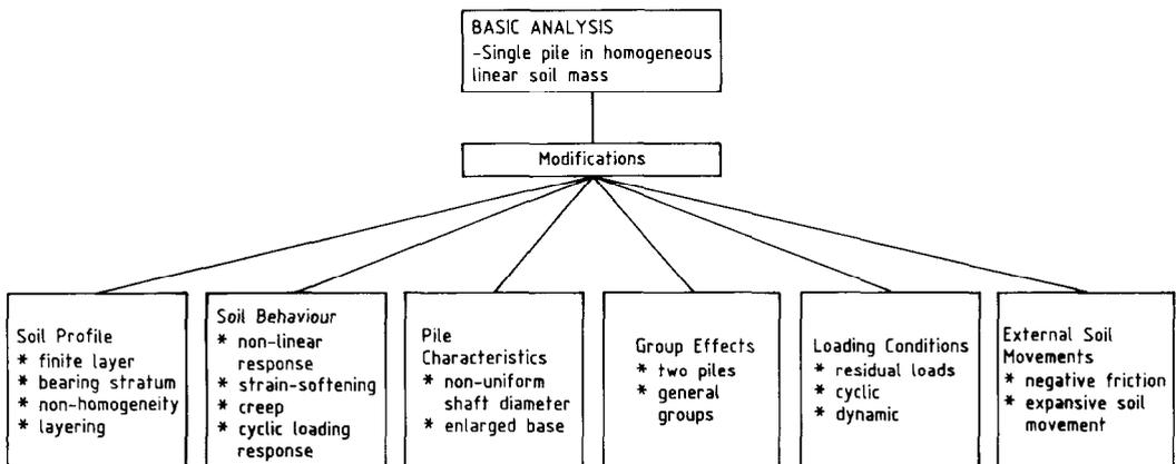
Fig. 2. Basic analysis, and extensions to allow for more realistic modelling
