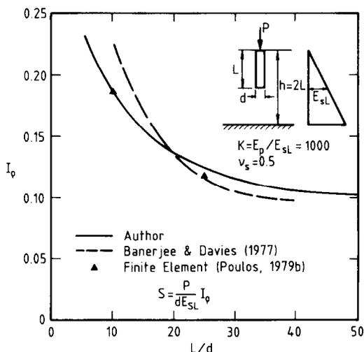
Fig. 4. Comparison between solutions for settlement of single pile in Gibson soil layer of finite depth
