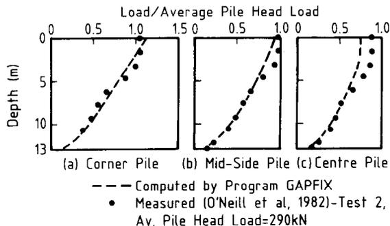
Fig. 49. Comparison between computed and measured load distribution in 9 pile group test
