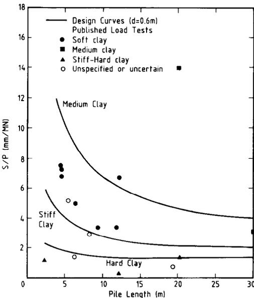
Fig. 33. Design chart for settlement of bored piles in clay (diameter =  $0.6 \pm 0.1$  m)
