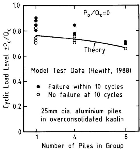
Fig. 24. Influence of number of piles on failure under two-way cyclic loading
