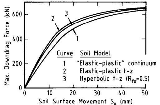
(a) Max. Dowdrag Force vs. Soil Surface Movement
