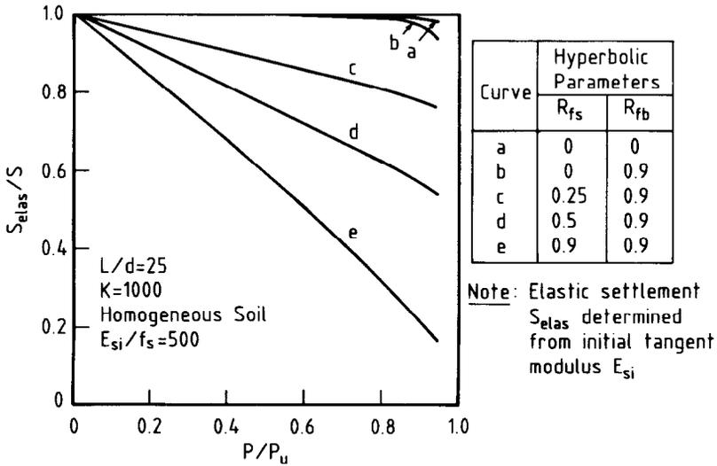
**Fig. 11. Example of influence of nonlinearity on computed pile settlement. Hyperbolic interface model**
