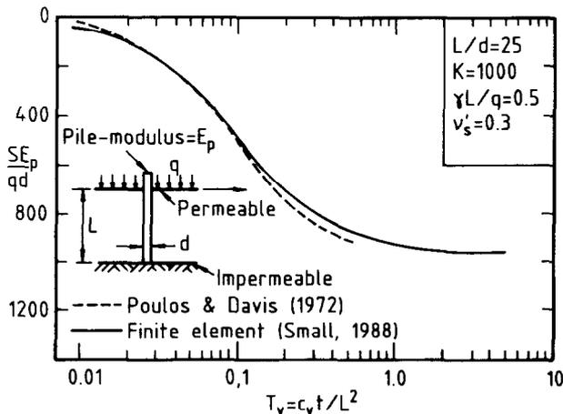
Fig. 7. Vertical deflection of pile head with time
