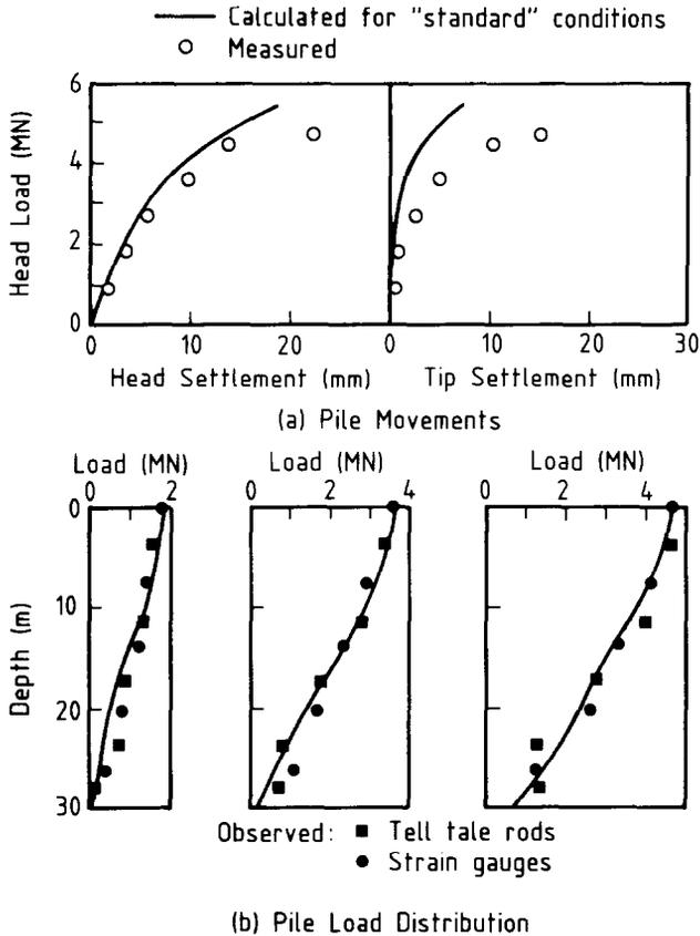
Fig. 41. Comparisons between observed and theoretical behaviour, pile test A (Gurtowski & Wu, 1984): (a) pile movements; (b) pile load distribution
