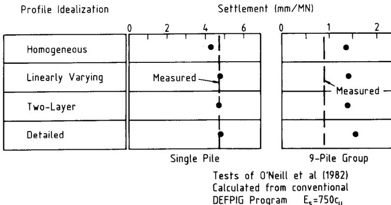
Fig. 50. Effect of soil profile idealization on single pile and group settlements
