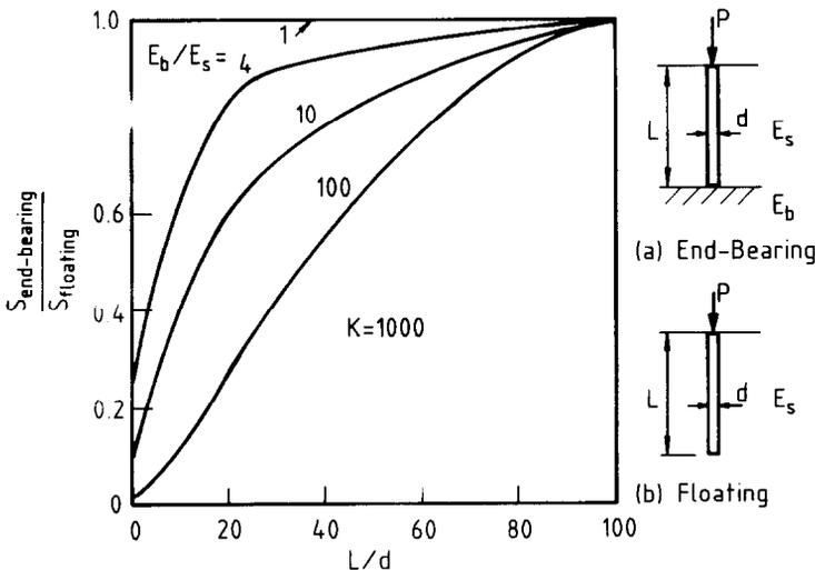
Fig. 9. Relative settlement of end bearing and floating pile. Homogeneous soil
