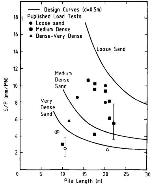
Fig. 34. Design chart for settlement of bored piles in sand (diameter =  $0.5 \pm 0.1$  m)
