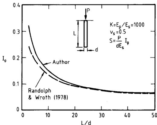
**Fig. 3. Comparison between solutions for settlement of single pile in deep uniform elastic soil layer**
